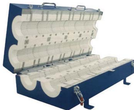
Twin-Parallel Tube Furnace: Used in an electronics plant. Furnace featured two heating chambers, each 6" (0.15m) inside diameter by 54" (1.37m) long. Operating temperature is 2200°F (1200°C). Includes internal support blocks for quartz tubes.
