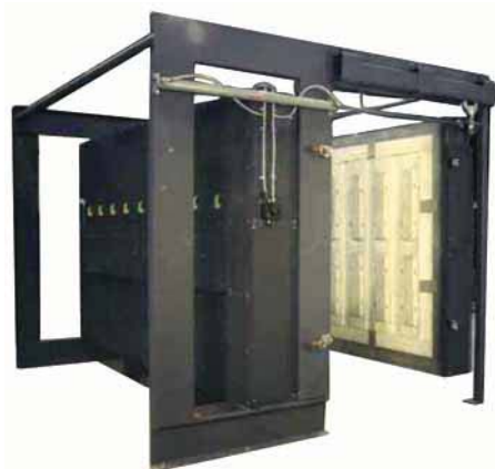
Ethylene Cracking Furnace: This furnace was designed as part of a petrochemicals pilot plant. Chamber is 78" (1.98m) wide by 60" (1.52m) high by 10" (0.25m) deep. Operating temperature is 2200°F (1200°C). Furnace features pneumatic sliding door.
