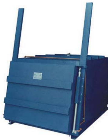
Box Furnace: For annealing, hardening, tempering, and general heat treating. Chamber is 30" (0.76m) wide by 30" (0.76m) high by 48" (1.21m) deep. Operating temperature is 2200°F (1200°C). Furnace featured air-assisted vertical lift door.
