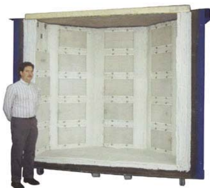
Cell Furnace: Large split furnace designed for heating vats of liquid. Chamber is 89" (2.26m) inside diameter by 82" (2.08m) high. Operating temperature is 1800°F (980°C). Furnace is supported on a sliding rail system for easy loading and unloading.
