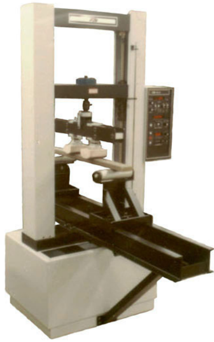
Series 1120C UTM integrated with a 60" span bend test fixture. Used for static testing of timbers per ASTM designation D198-84.
