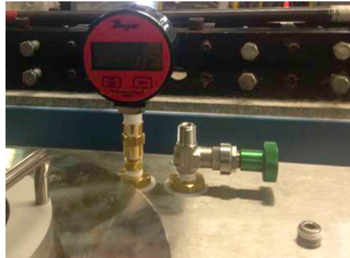
Figure E.7 - Pressure vacuum gauge attached
