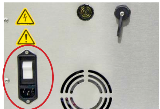
Figure D.2 - AC Power Connection and ON/OFF Switch
