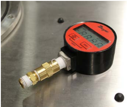
Figure E.6 - Brass extension fitting on gauge
