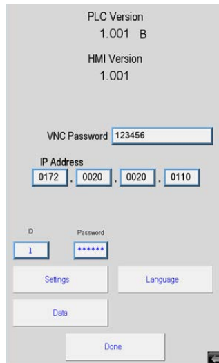
Figure E.8 - View Screen without Engineering button
