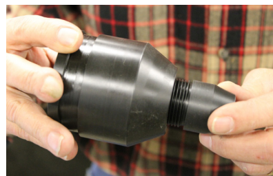
Figure D.3 - Unscrew the Lower Portion of the Load Shroud
