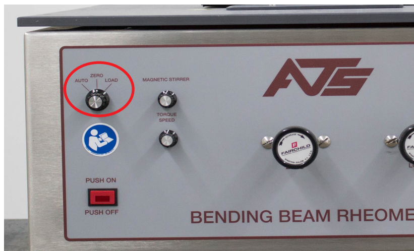
Figure E.12 - Load Control Switch
