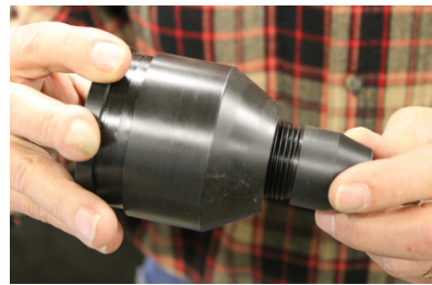
Figure D.3 - Unscrew the Lower Portion of the Load Shroud
