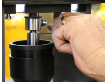
Figure D.5 - Tightening the Set Screw
