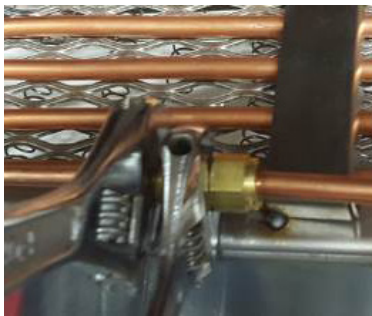
Figure H.12 - Loosen the nuts on the air line feed.
