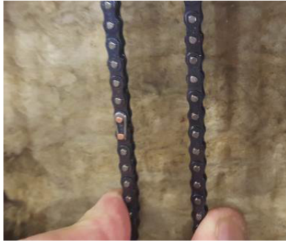
Figure H.10 - Check the chain for proper tension.
