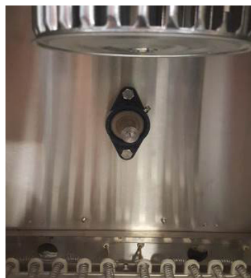
Figure H.9 - Front inside bearing exposed.
