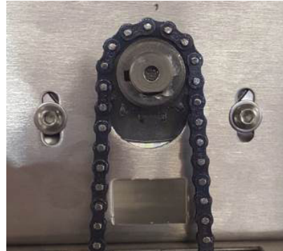
Figure H.11 - Checking the set screws on the top sprocket.
