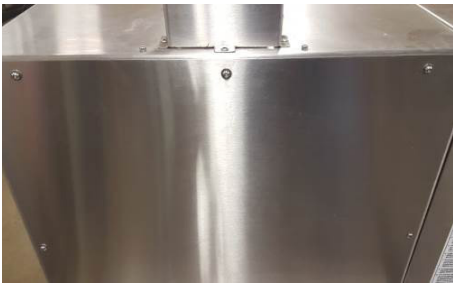
Figure H.1 - Remove the five screws for the chain guard.
