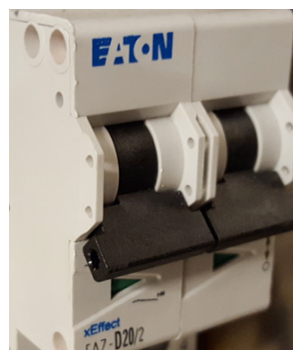
Figure G.1 - Circuit breaker in the “OFF” position
