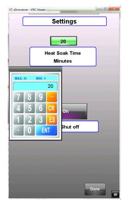
e. The heaters on the PAV can be set to automatically shut off once a test is completed. Select "On" for this option. Selecting "Off" will cause the heaters to continue running after a test is complete.
