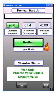
Once the PAV has reached the setpoint, the display will prompt the operator to insert the specimens, secure the lid, and select "Age."
