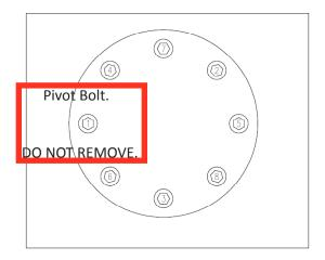
g. Slide the vessel lid closed and insert bolts. The bolts only need to be engaged a turn or two. It is not necessary at this time to completely tighten the bolts. Close the oven lid and secure using the latches. h. Select "Off" from the "Preheat Startup" screen to start the preheating process. When the PAV is heating, the Heat Mode will display "Heating" and a flame symbol will appear.
