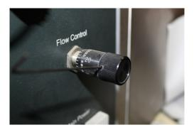
6. Turn the valve slowly counter-clockwise to open. Each full rotation should equal one line on the barrel. Rotate the knob to the value recorded on the calibration sticker. If there is no value on the calibration sticker, the default value is 10.
