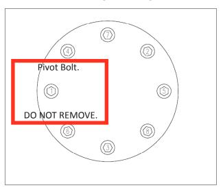
vi. Tighten in sequential order with the wrench provided. Go around twice to tighten bolts to 55 inch/pounds.
