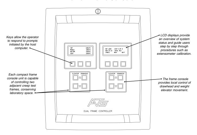
The frame console is an integral component of the WinCCS II system and is a major innovation in multiple-frame creep testing. The console displays step-by-step instructions from the host computer for procedures such as extensometer calibration and specimen loading. Keys are provided for the operator to respond after each step. During testing, critical information such as temperature and creep rate is available at a glance.
