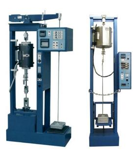
▲ Lever arm and direct load test frames, any number and in any combination, from any manufacturer, can readily be adapted to suit the WinCCS II system. WinCCS II can also be supplied as an integral part of a new ATS creep testing installation.
