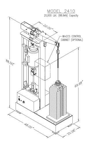
Model 2410 Lever Arm Test System shown in a typical creep testing setup, including dual-ratio lever arm, calibrated load weights, alignment couplings, split tube furnace, automatic beam-leveling drawhead, and computerized hot step loading via WinCCS software.
