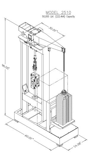
Model 2510 Lever Arm Test System shown in a typical creep testing setup, including single-ratio lever arm, calibrated load weights, alignment couplings, custom metals testing extensometer, electric weight elevator, and manual control station.
