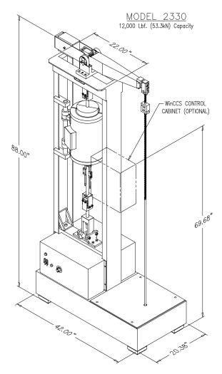
Model 2330 Lever Arm Test System shown in a typical creep testing setup, including single-ratio lever arm, alignment couplings, split tube furnace, averaging extensometer, automatic drawhead drive system, and automatic (weightless) loading via WinCCS software and drawhead drive.
