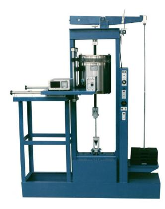
Special Series 2330 Lever Arm Creep Tester designed for tensile testing of ceramic specimens. Features include a high-temperature furnace and integrated slide table for use with non-contacting laser extensometer.
