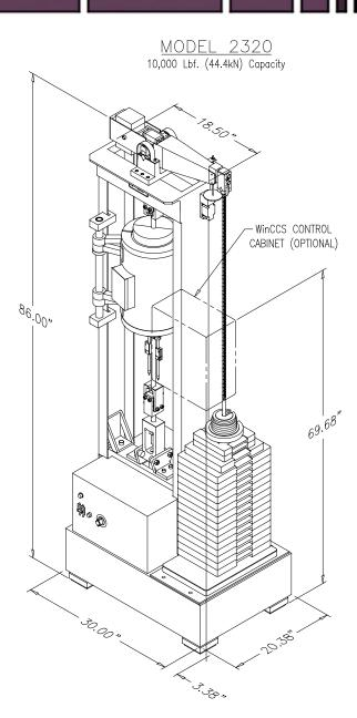
Model 2320 Lever Arm Test System shown in a typical creep testing setup, including single-ratio lever arm, calibrated load weights, alignment couplings, split tube furnace, averaging extensometer, and automatic beam-leveling drawhead.
