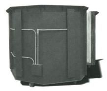
Large split pit furnace, 1800°F (982°C), 74" (1.8m) diameter, 82" (2.1m) deep, built for a specialty metals manufacturer
