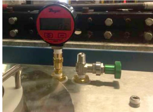
Figure E.7 - Pressure vacuum gauge attached
