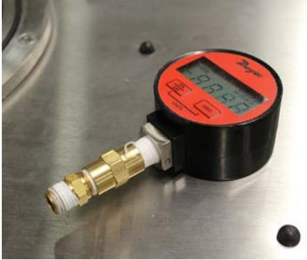
Figure E.6 - Brass extension fitting on gauge
