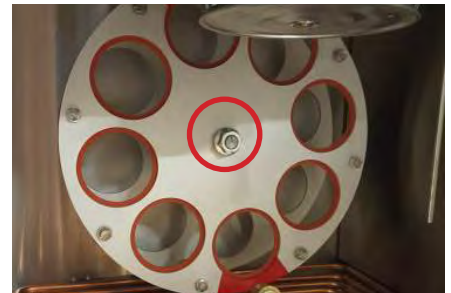
Figure H.6 - Front inside bearing set screw
