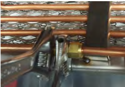
Figure H.4 - Loosen nuts on the air line.
