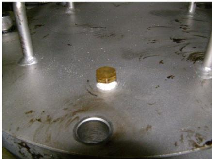
2. Screw the pressure gage into that space. Make sure the lid is secured according to the directions in Section 5.
