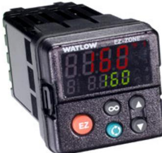
3. Press the bottom two buttons simultaneously (the Advance key and the Down key) for three seconds until the digital display shows COM in the upper display and rUi in the lower display. The communication menu should appear.
