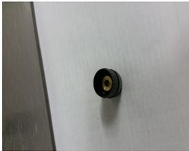
3. Rotate the shaft fully clockwise to close the flow adjust valve.
