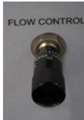
Figure D.4: Flow Control valve
