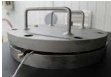
Figure G.4 - Keep lid from pinching wire
