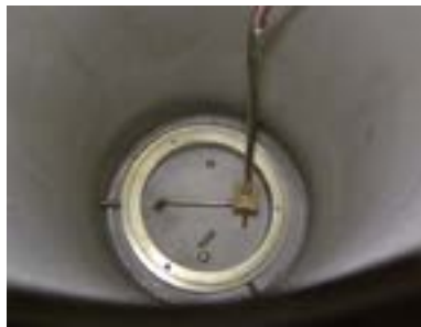
Figure G.3 - Calibration block on RTD
