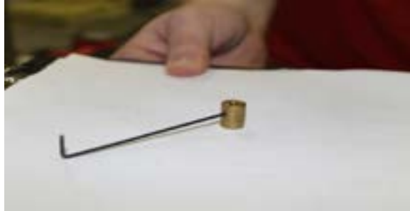
Figure H.3 - Tighten with Hex Wrench
