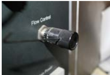
Figure H.4 - Turn Valve Counter-Clockwise
