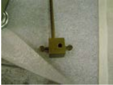
Figure G.1 - Temperature Probe inside Calibration Block
