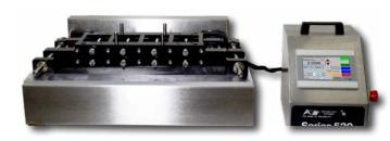
Line of equipment designed to simulate the expansion and contraction of sealant joints under extreme environmental conditions.
