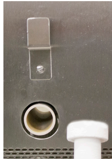
Ceramic tube port for thermocouples during temperature survey. When not in use, an insulating plug is supplied.
