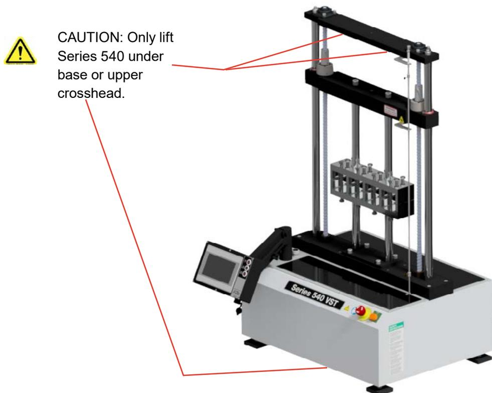
Figure D.1: Lifting Series 540 Sealant Tester
