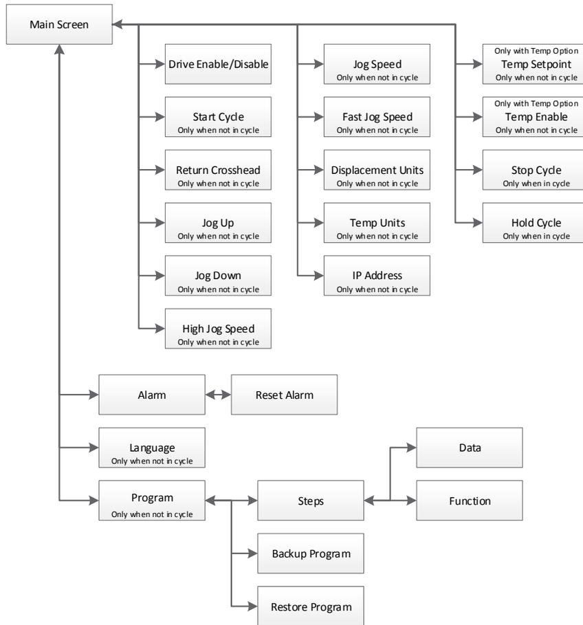
Figure E.1: Series 540 Sealant Tester Software Map
