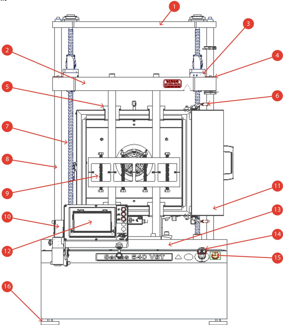
Figure C.1.: Series 540 Sealant Tester (Front View)
