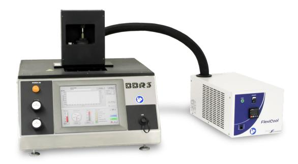
The ATS Bending Beam Rheometer 3 (BBR3) performs flexural tests on asphalt/bitumen binder and similar specimens per AASHTO T 313, AASHTO TP 87, ASTM D6648, and BS EN 14771 specifications as part of the PG grading system according to Superpave. An ATS original, the BBR3 is the first of its kind to offer a state of the art internal computer system, incorporating intuitive new software and touchscreen technology.
