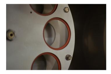
Silicone rings allow for easy install and prevent damage to bottles.
