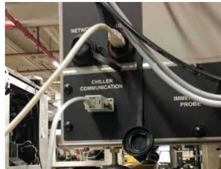
Figure D.12 - Chiller Communication Cable in BBR3 Chiller Communication Port
