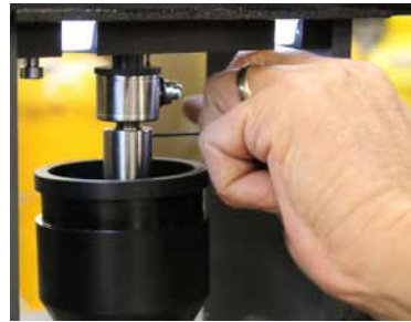
Figure D.4 - Tightening the Set Screw
