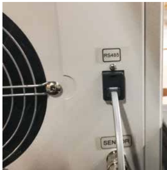
Figure D.11 - Chiller Communication Cable in RS-485 Port
