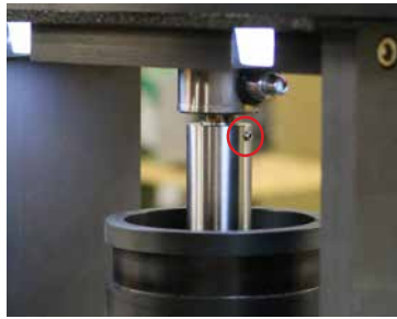
Figure D.3 - Set Screw Location on Load Nose
