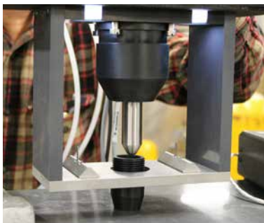
Figure D.6 - Attaching Lower Portion of Load Shroud
