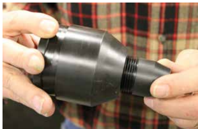
Figure D.2 - Unscrew the Lower Portion of the Load Shroud
