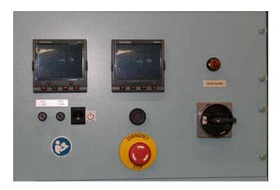
If the controller is equipped with an emergency stop button (E-stop button), be sure it is functioning properly by pushing the knob (this will stop the test in an emergency) and then pulling the knob and rotating it according to the arrows on the knob (this will re-engage the E-stop).
