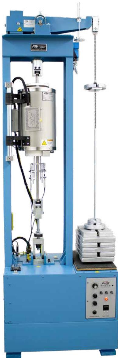
**Creep/Stress Rupture Tester**
