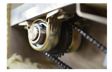
Sealed high temp bearings located outside of heat zone for zero maintenance & durability.
