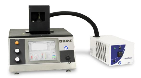
The ATS Bending Beam Rheometer 3 (BBR3) performs flexural tests on asphalt/bitumen binder and similar specimens per AASHTO T 313, AASHTO TP 87, ASTM D6648, GOST 58400.8-2019, and BS EN 14771 specifications as part of the PG grading system according to Superpave. An ATS original, the BBR3 is the first of its kind to offer a state of the art internal computer system, incorporating intuitive new software and touchscreen technology.
