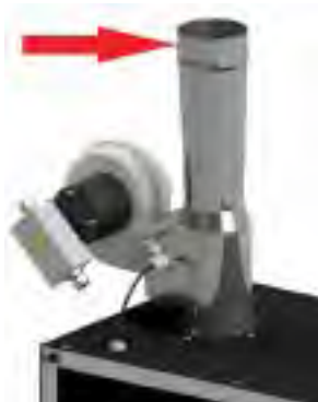
Figure D.4: Attach a 6"-8" section of flexible duct to the 4" OD Draft Inducer Outlet using a 4"-6" transition adapter.
