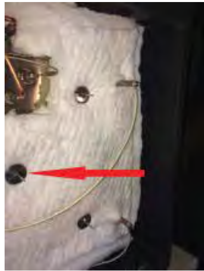
Figure H.8: Heating element connections & insulation retainers (5)
