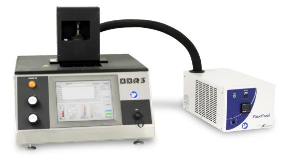
The ATS Bending Beam Rheometer 3S (BBR3S) performs flexural tests on asphalt/bitumen binder and similar specimens per AASHTO T 313, AASHTO TP 87, ASTM D6648, GOST 58400.8-2019, and BS EN 14771 specifications as part of the PG grading system according to Superpave. An ATS original, the BBR3S is the first of its kind to offer a state of the art internal computer system, incorporating intuitive new software and touchscreen technology.
