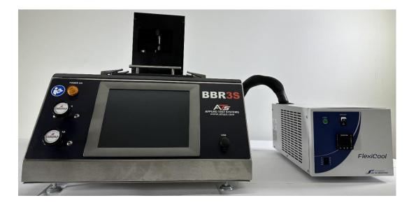
The ATS Bending Beam Rheometer 3S (BBR3S) performs flexural tests on asphalt/bitumen binder and similar specimens per AASHTO T 313, AASHTO TP 87, ASTM D6648, GOST 58400.8-2019, and BS EN 14771 specifications as part of the PG grading system according to Superpave. An ATS original, the BBR3 is the first of its kind to offer a state of the art internal computer system, incorporating intuitive new software and touchscreen technology.
